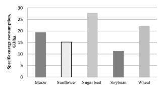
Fig. 1 Specific energy consumption in crop production
